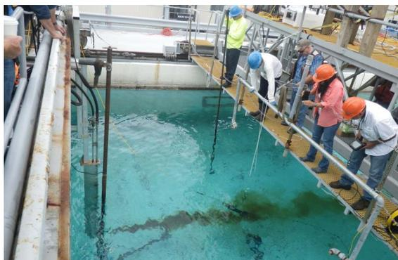
Figure 1. Subsurface oil release over AZFP.
